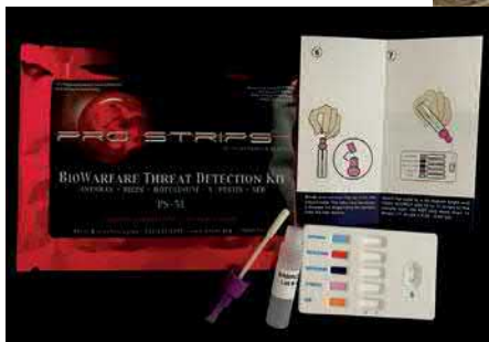
Pro Strips Rapid Screening System, developed by ADVNT Biotechnologies LLC, is the first advanced multi-agent biowarfare detection kit that tests for anthrax, ricin toxin, botulinum toxin, plague, and SEB (staphylococcal enterotoxin B).
